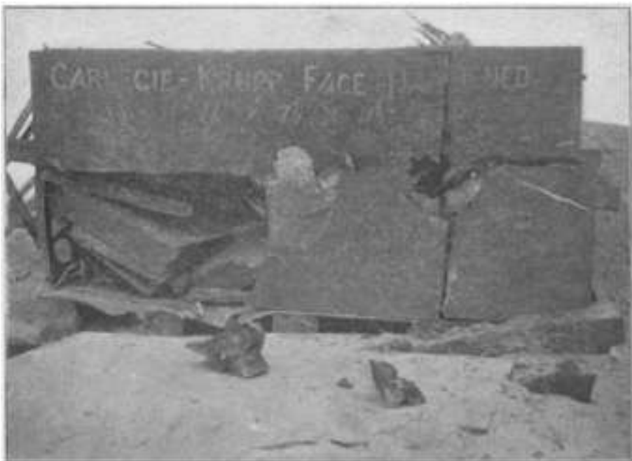
An 11 \frac{1}{2} -inch Kruppized Plate After Attack by Three of Our 12-Inch Armor-Piercing High-Explosive Projectiles. Plate and Backing Completely Wrecked.
