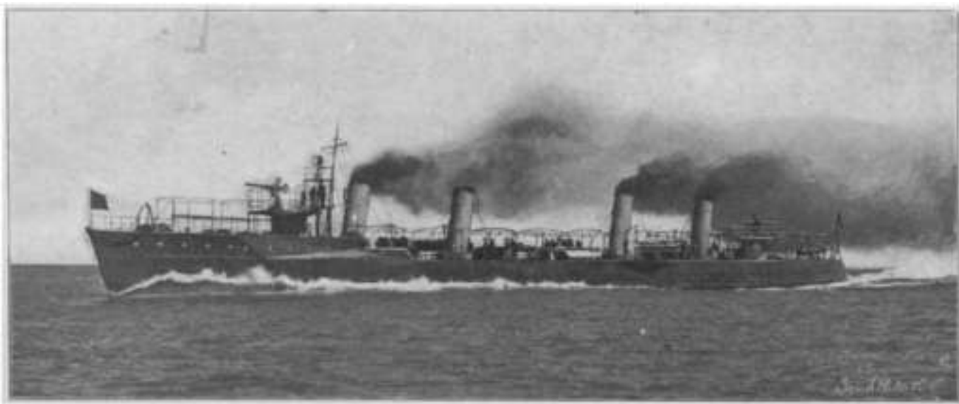
Length, 245 feet. Breadth, 23 feet 7 1/4 inches. Draft, 6 feet 6 inches. Displacement, 420 tons. Contract Speed, 29 knots. Bunker Capacity, 139 tons. Armament: Two long 18-inch Whitehead torpedo tubes; two 3-inch R. F. guns; five 6-pounders. Complement, 73.
