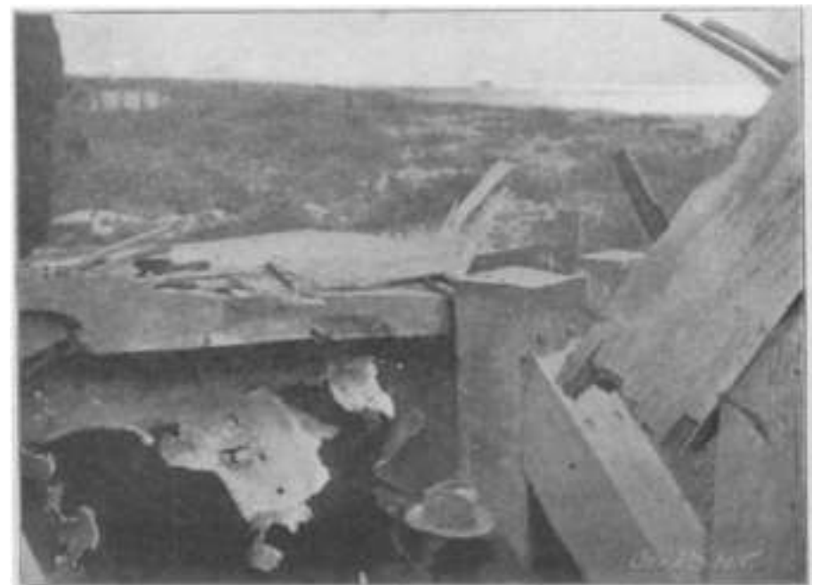
Rear View of Same Target, Showing Complete Destruction Wrought by 12-Inch Armor-Piercing Shot Loaded with 20 Pounds of the New Government High-Explosive.
