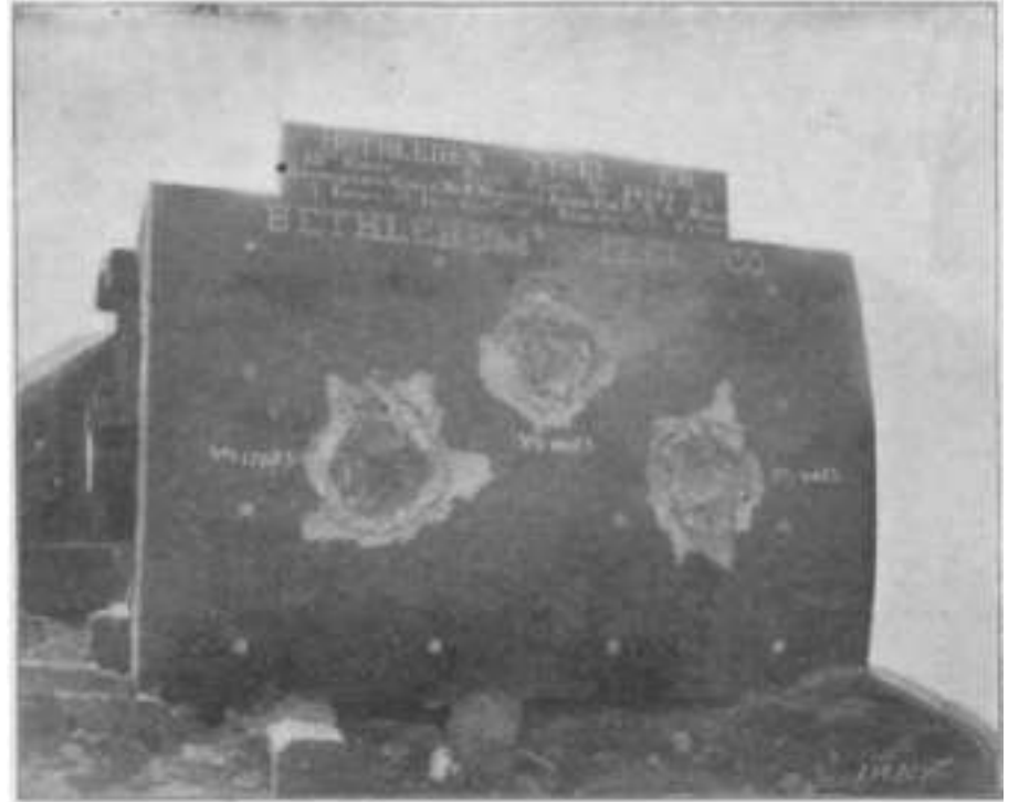
12-Inch Kruppized Armor Plate, Representing Armor for the "Maine," After Attack by Three 12-Inch Shells. Projectiles Smashed on Plate. Penetration, 6\frac{1}{2} Inches, 4\frac{1}{4} Inches, and 4\frac{1}{4} Inches.
